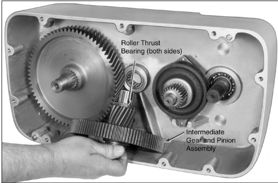
Figure 5-4. Removing Intermediate Gear and Pinion Assembly
